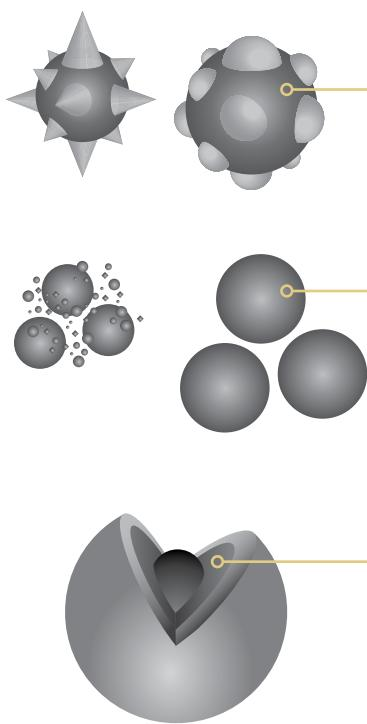
**Pre-attrition** is the process by which an activated carbon is subjected to force or attrition before it is sent to the customer site. This process breaks off sharp edges that would otherwise readily adsorb gold and be lost in screening, and reduces the initial degradation that the customer will see on site.
